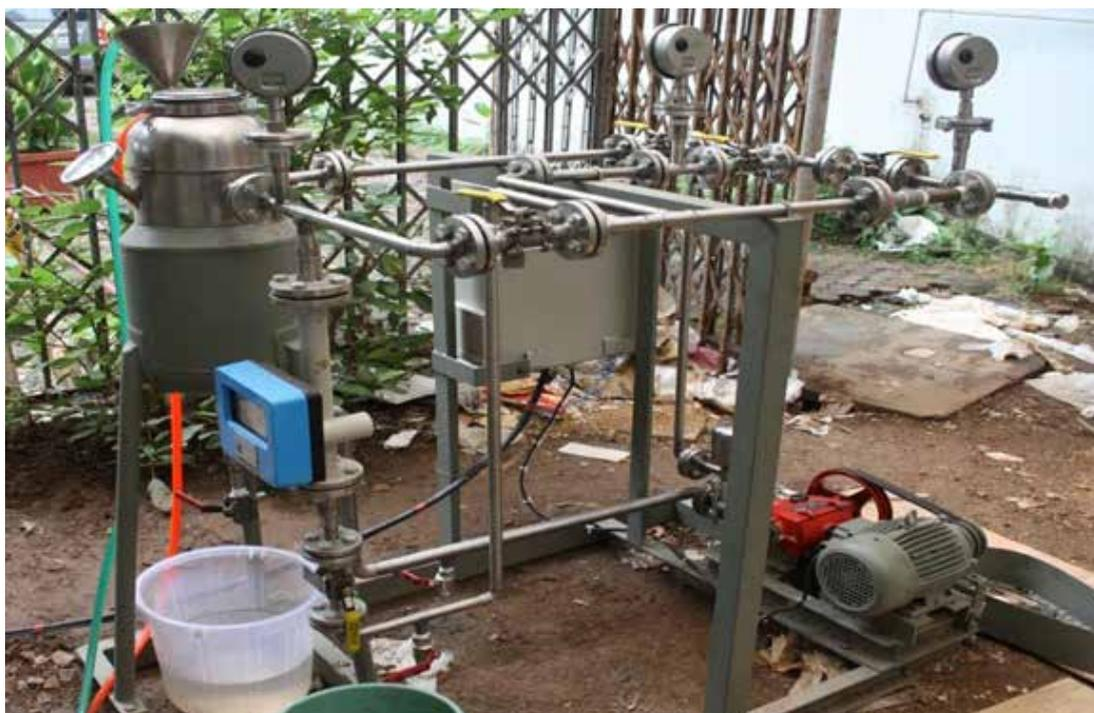
Hydrodynamic Cavitation Set-up
