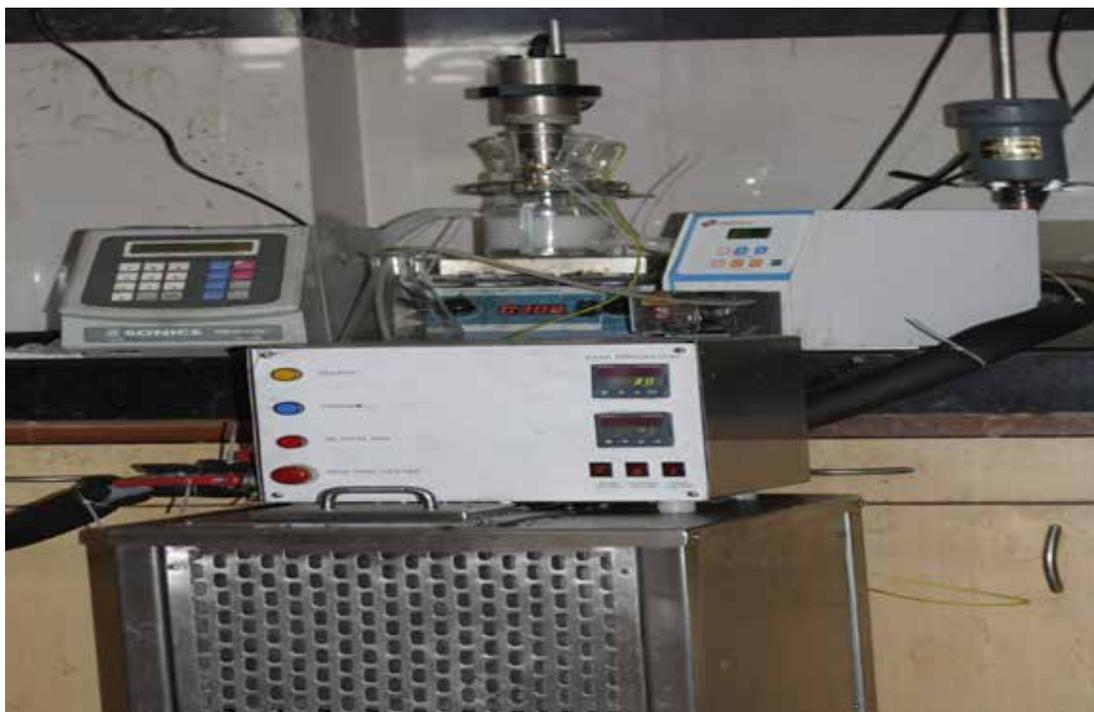
Acoustic cavitation set-up
